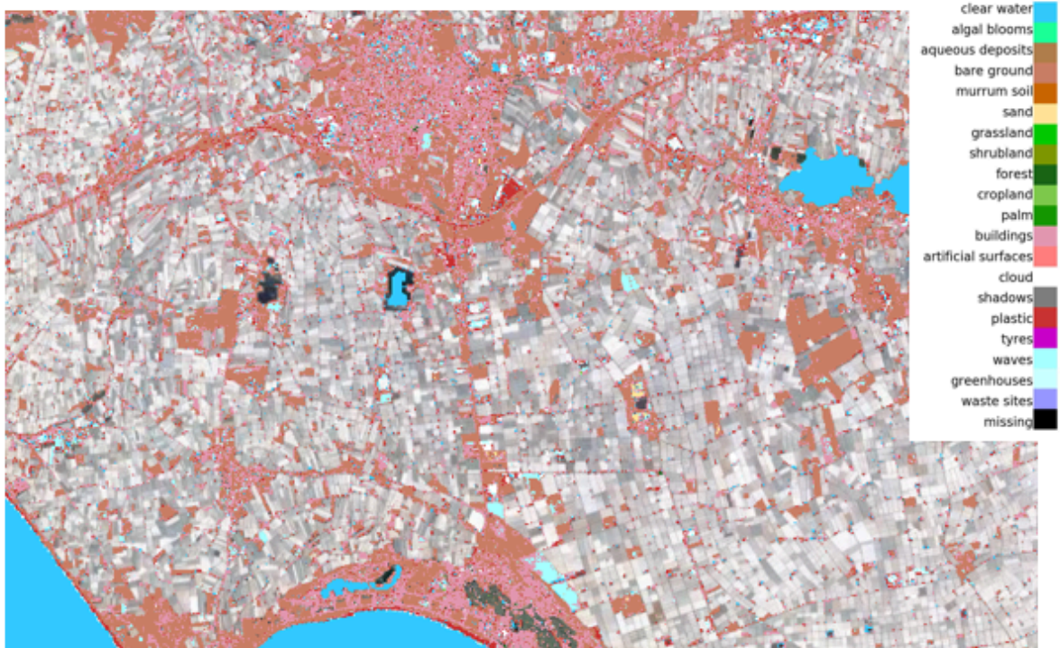
Figure 25 – Sentinel-2 NNet model output for the Almeria region in Spain with Transfer Learning applied.
