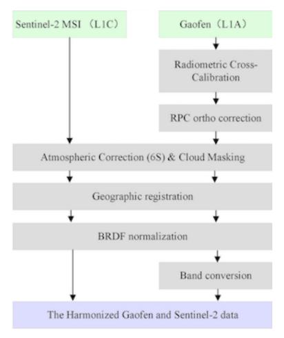
**Figure 41** – The processing chain to produce harmonized ARD.
