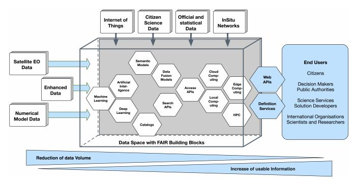
**Figure 4** — Schematic Architecture of a Climate Resilience Information System. By respecting FAIR principles for the climate application packages the architecture enables open infrastructures to produce and deliver information on demand of the users needs
