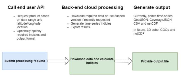
Figure 24 – Pixalytics drought severity workflow architecture
