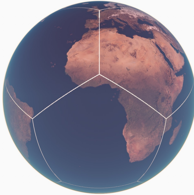
Figure 89. The dodecahedron (12 pentagonal faces) used as a starting point in these experiments (level 0)
