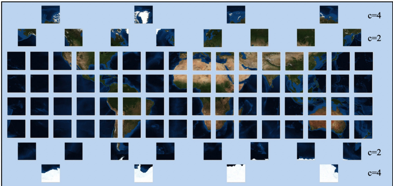
Figure 80. Tile Matrix (zoom level) 2 from the GNOSIS Global Grid 2D Tile Matrix Set, showing the different coalescence factors ( c ) for different latitude rows near the poles (OGC 17-083r4)
