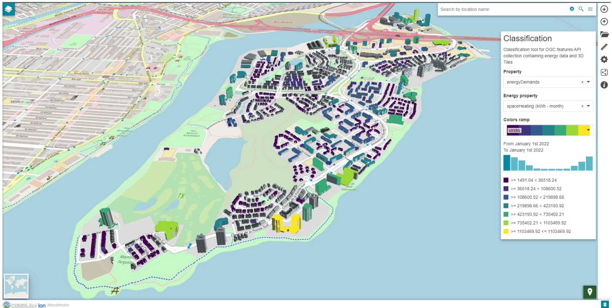
Figure 54 – Style classification based on monthly energy demand property applied to the interactive instruments's Nun's Island collection visualized in 3D inside a MapStore custom application
