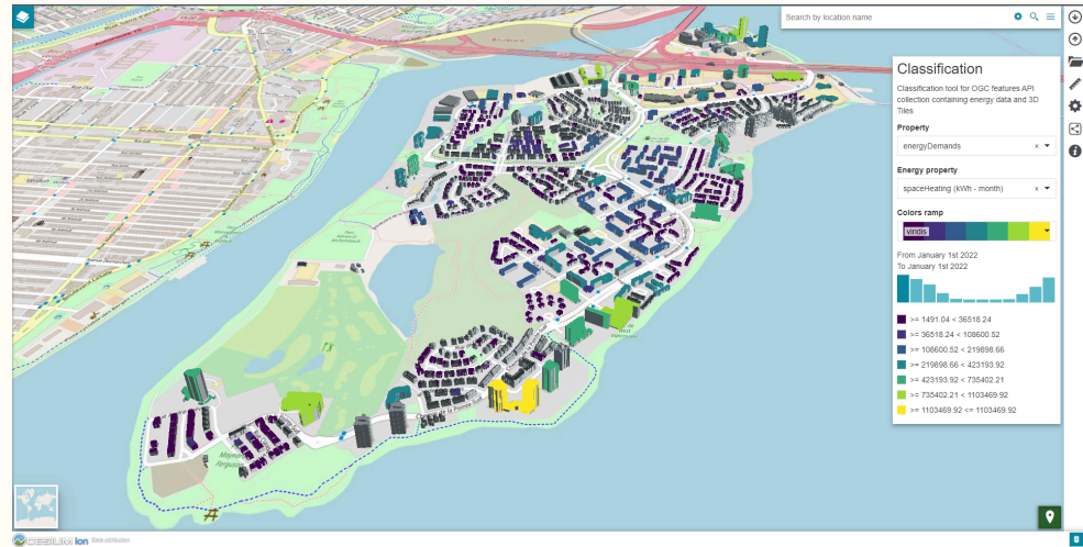
Figure 43 – Style classification based on monthly energy demand property applied to the interactive instruments's Nun's Island collection visualized in 3D inside a MapStore custom application
