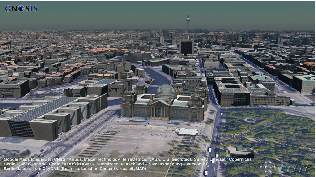
Figure 42. Textured dataset of Berlin originating from CityGML being served as 3D Tiles by virtualcityMAP from virtualcitySYSTEMS (additional non-participating service tests)
