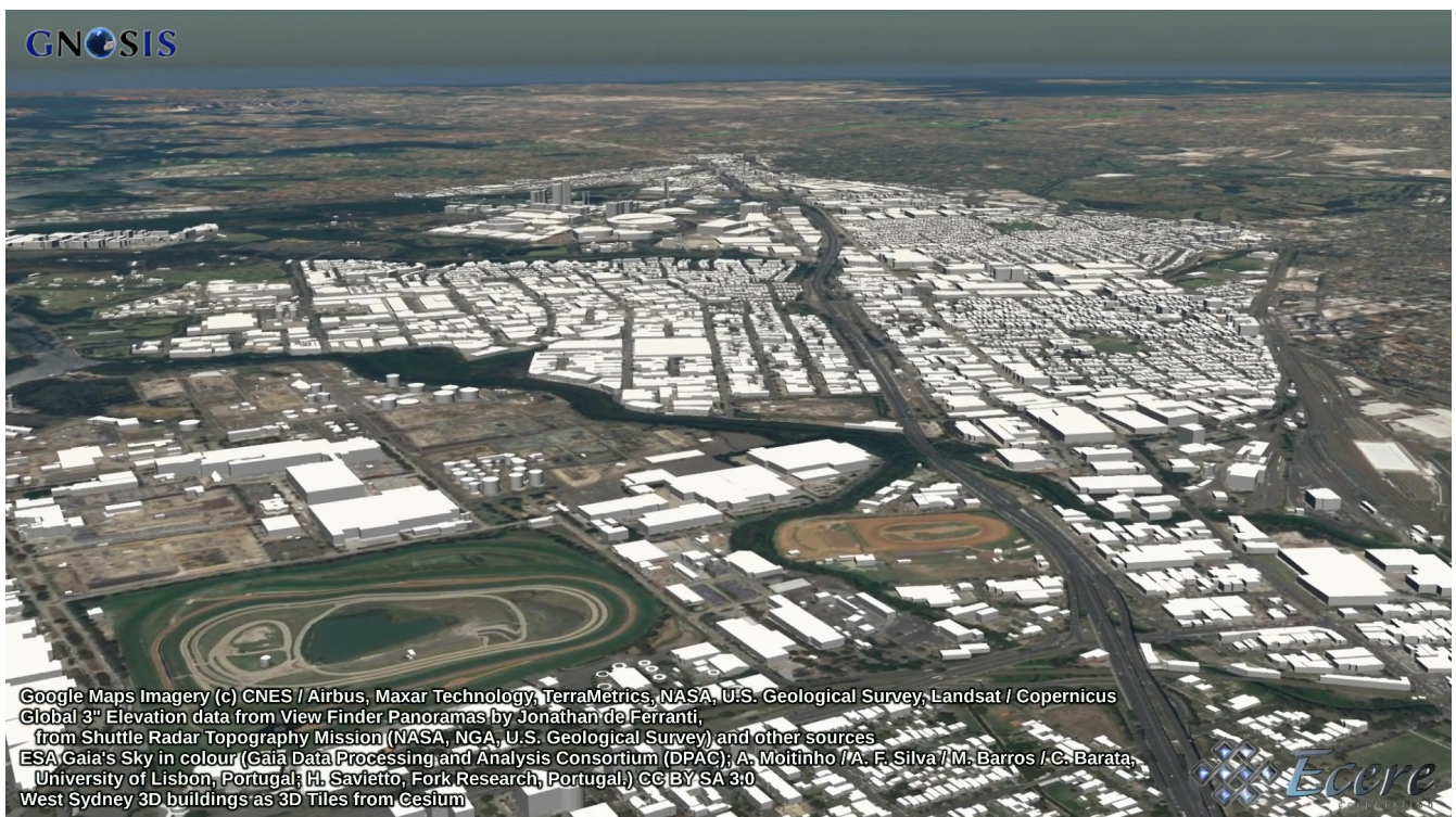
Figure 45. 3D buildings of West Sydney accessed as 3D Tiles from Cesium service (larger buildings)
